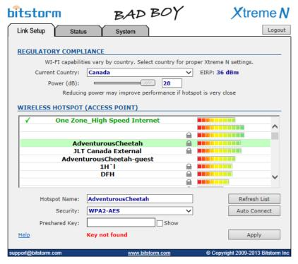
applied. The Preshared Key will be saved internally and automatically used on subsequent connections to this hotspot. The Auto Connect button will cause Xtreme to connect to the strongest unsecured signal that it finds. Keep in mind that the strongest signal may not always be your best choice when using a public hotspot.
